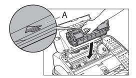
Insert the toner cartridge so that the guide (A) on the left side of the toner cartridge fits into the groove inside the machine and slide it down parallel to the guide.
